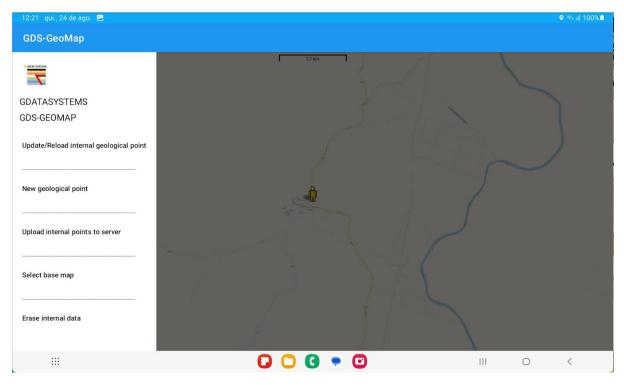
Selecting New geological point will bring the following form to be completed accordingly. The latitude, longitude and elevation values are extracted from the tablet GPS at the location when the menu item is pressed.
